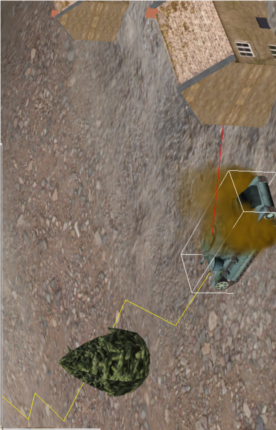
Figure 6.2: An animated character - in this case a to-scale model of a Soviet T-28 circa 1932 with simulated real physical operating characteristics - travels through a 3D-environment in the simulation engine complete with hills and a range of obstacles. The vehicle has planned a prospective path around obstacles using the A* component of the Hybrid Fuzzy A* algorithm (as indicated by the segmented line visible ahead of the vehicle in the figure) and has detected and is driving around the nearest obstacle on its right hand side (as indicated by the second line visible in the Figure) - in this case a house.
