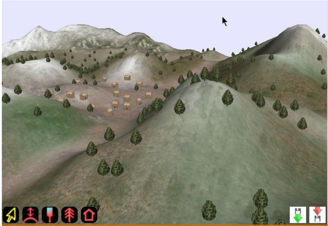
Figure 4.5: User-assisted dynamic landscape generation. Pictured is a real-time tool for deforming a 3D landscape into a desired experiment scenario by using the mouse to “drag” hills up and valleys down. The diameter and shape of depressions and hills is adjusted via the user-interface buttons. The tool can also place, rotate, and adjust environment elements and obstacles onto the landscape, and generate large randomised arrangements of obstacles to quickly create scenarios for motion-control experiments.
