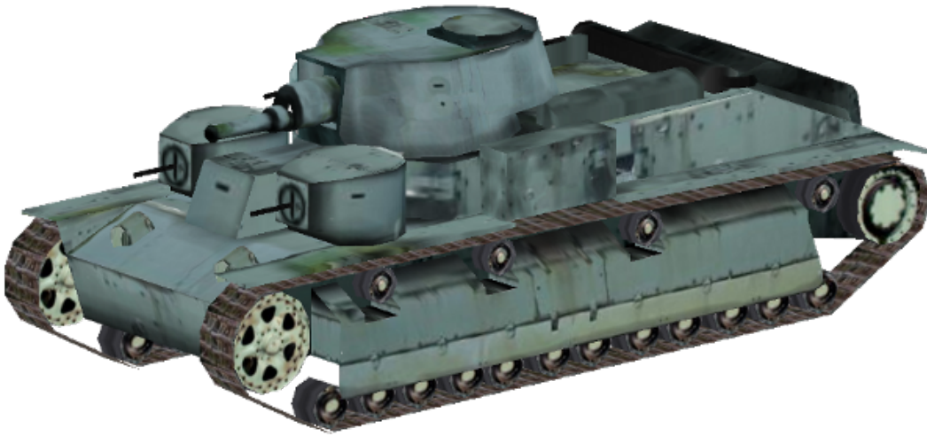
Figure 9.2: The to-scale 3D model of the T-28E vehicle with continuous tracks that was constructed for use in the experiment. This is a good example of an animated vehicle that would be reconstructed for a movie production or modern computer game or simulation. All of the historical performance data is available for this vehicle, and speed, weight, tracked steering movement and other available data is simulated.
